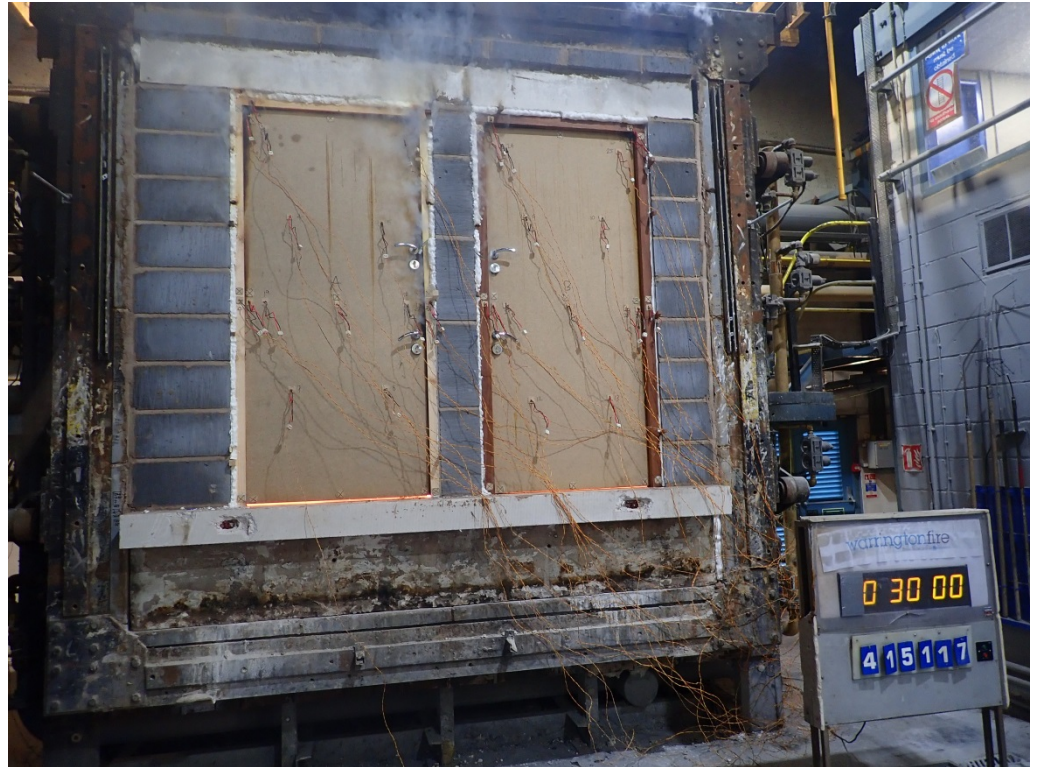
The unexposed face of the doorsets after a test duration of 30 minutes
