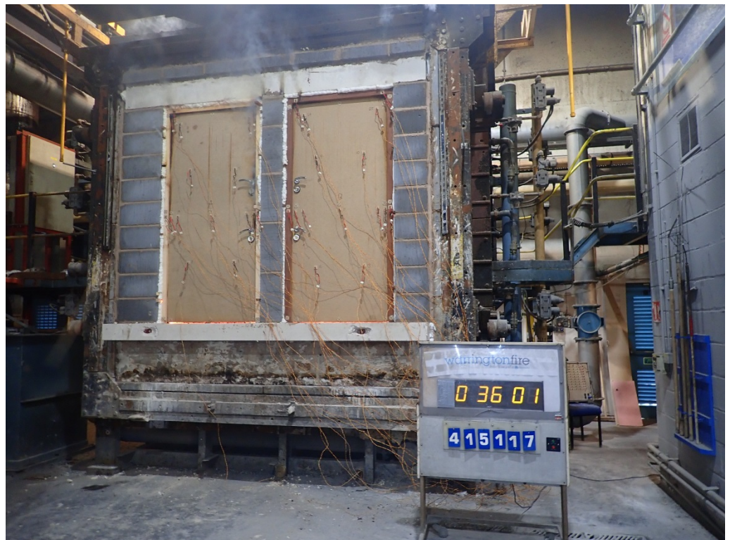
The unexposed face of the doorsets after a test duration of 36 minutes
