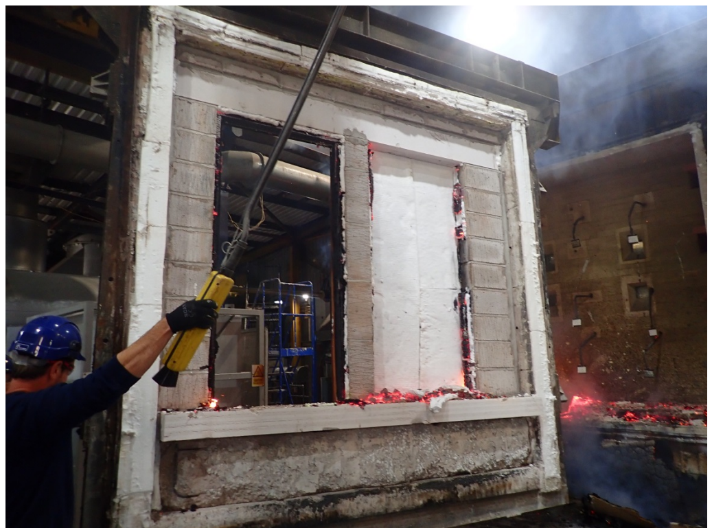
The exposed face of the test assembly shortly after the test
