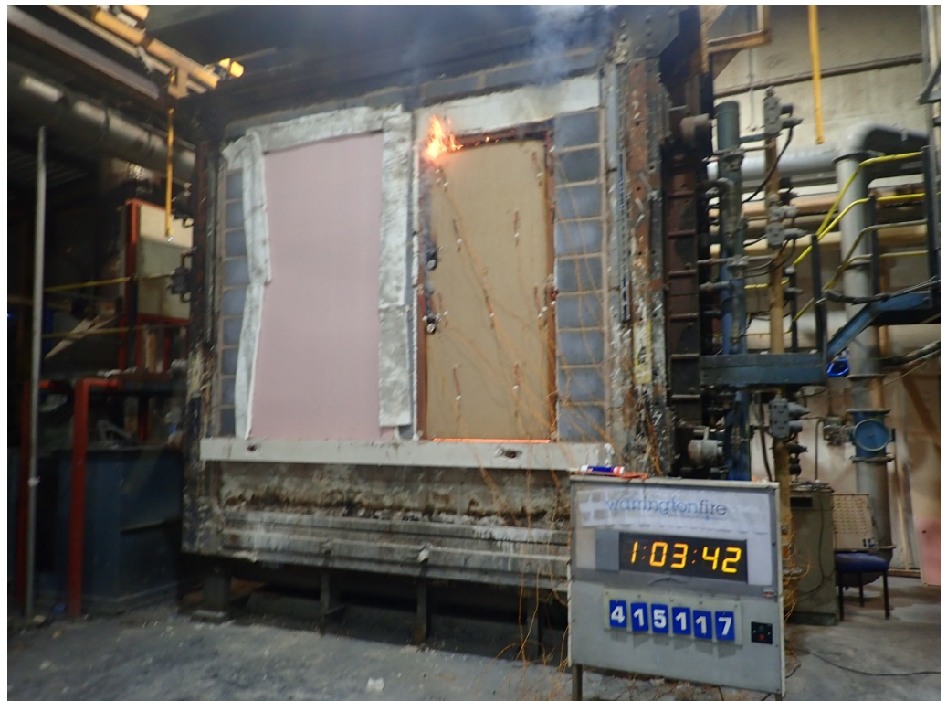
The unexposed face of Doorset B after a test duration of 63 minutes
