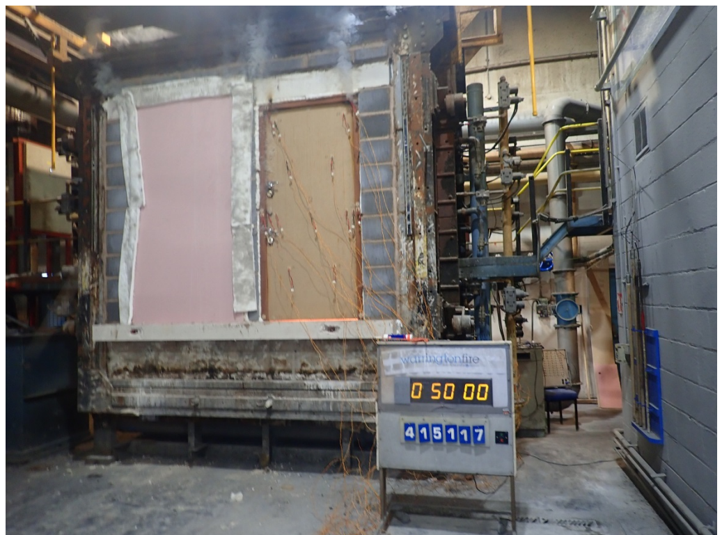
The unexposed face of Doorset B after a test duration of 50 minutes
