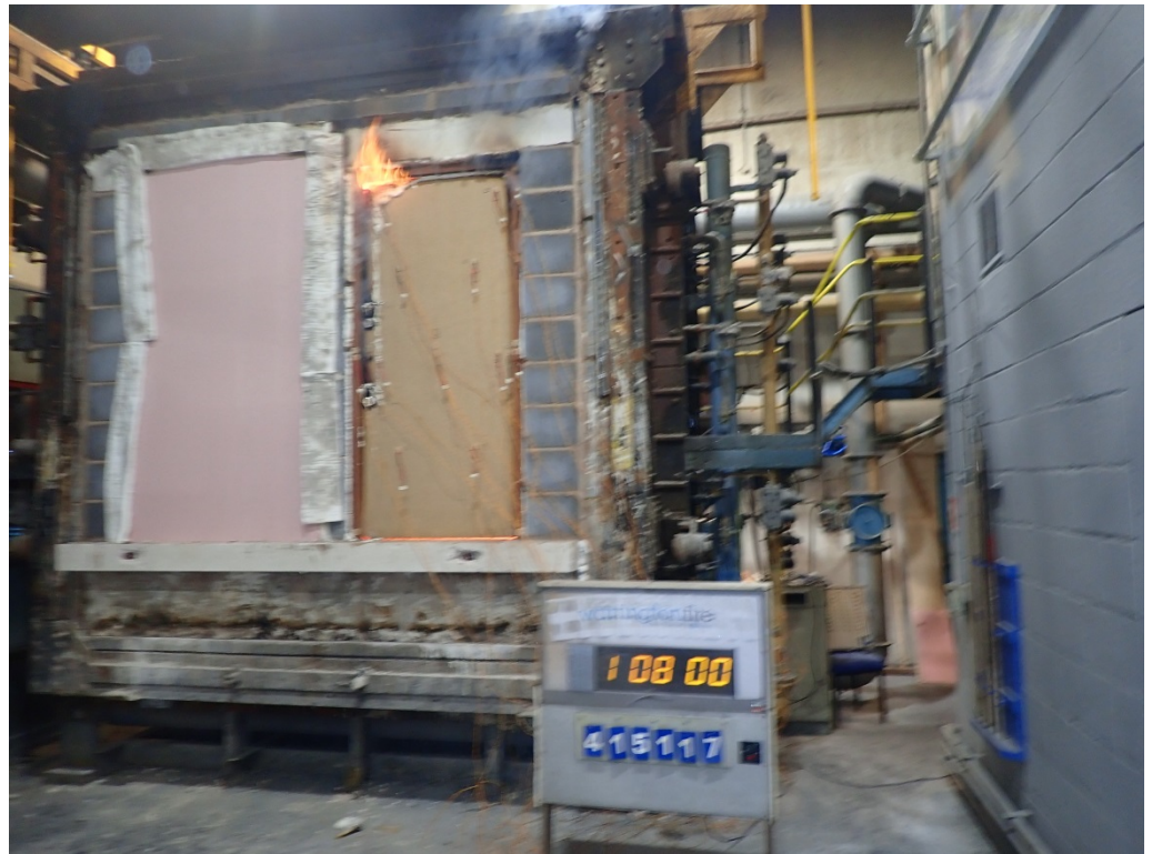
The unexposed face of Doorset B after a test duration of 68 minutes
