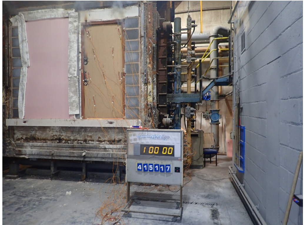
The unexposed face of Doorset B after a test duration of 60 minutes
