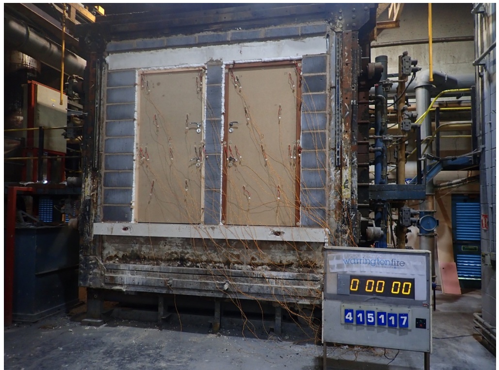
The unexposed face of the doorsets prior to the start of the test
