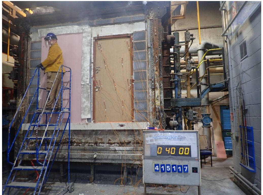
The unexposed face of Doorset B after a test duration of 40 minutes
