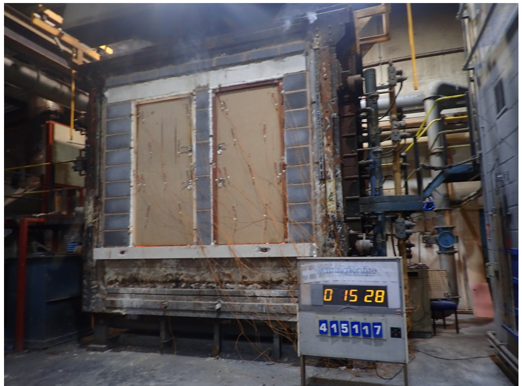
The unexposed face of the doorsets after a test duration of 15 minutes
