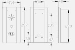
Stylish curved architectural model. Constructed from BS316 marine grade stainless steel and finished with gloss black acrylic trim. Complete with blue illuminated push button and integrated Prox reader. Kits complete with 3 proximity cards with additional cards available to purchase.
